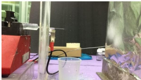
**Figure 1.** Experimental set up during electrospinning process.
