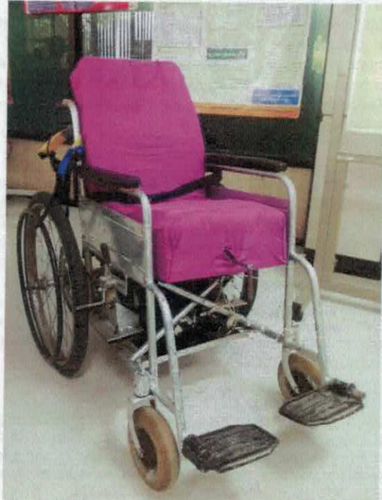
Fig. 6 shows the add-on seat attached to a wheelchair through a set of belts and straps.
