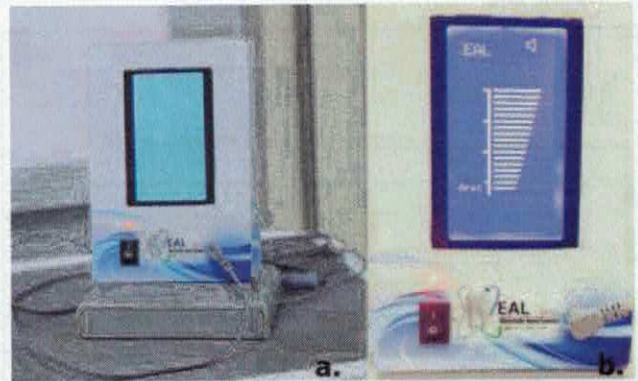
Fig. 8. Electronic Apex Locator; a. the whole device and b. the screen showed the depth of the file tip when it reached to the apex
